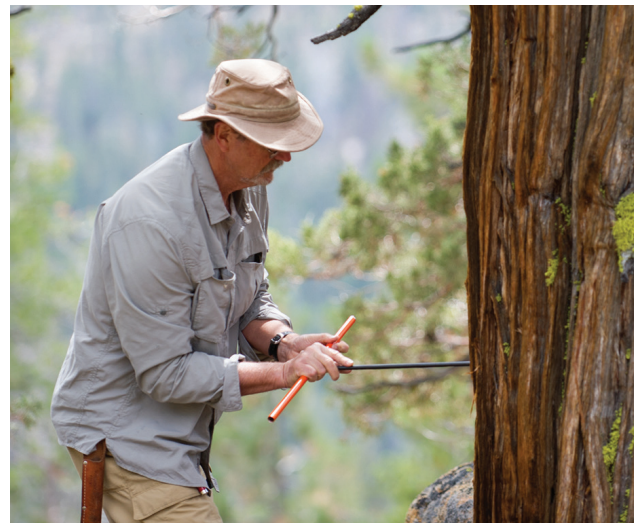
Collecting a tree-ring sample near Ebbetts Pass. Data from multiple trees at one site are combined into a single record representative of the site.
